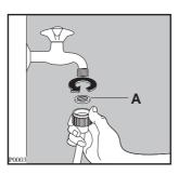
If only a cold water supply is available, connect the two hoses to a cold water outlet by means of a  ${}^{\times}Y{}^{\times}$  connection piece.
